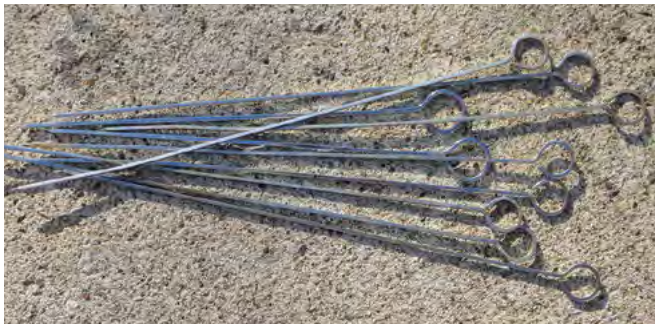
Kabob skewers for holding up marking tape.
